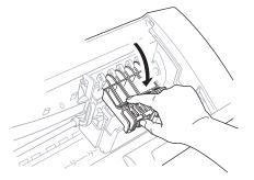
11 After installing the ink cartridges, close the top cover. Your MFC prepares for a "head cleaning" and goes online. The display screen prompts you to verify a new ink cartridge was inserted for each color you removed. Example: DID YOU CHANGE BLCK 1. YES 2. NO.
